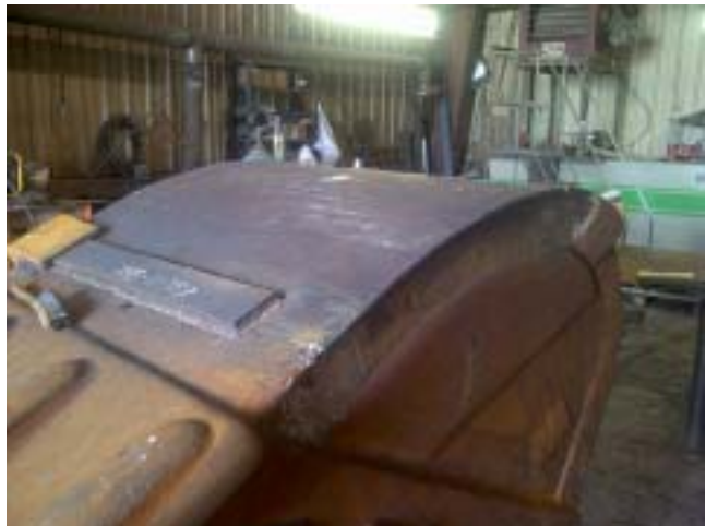
Excavator Rebuild with STULZ-CREUSABRO 4800
