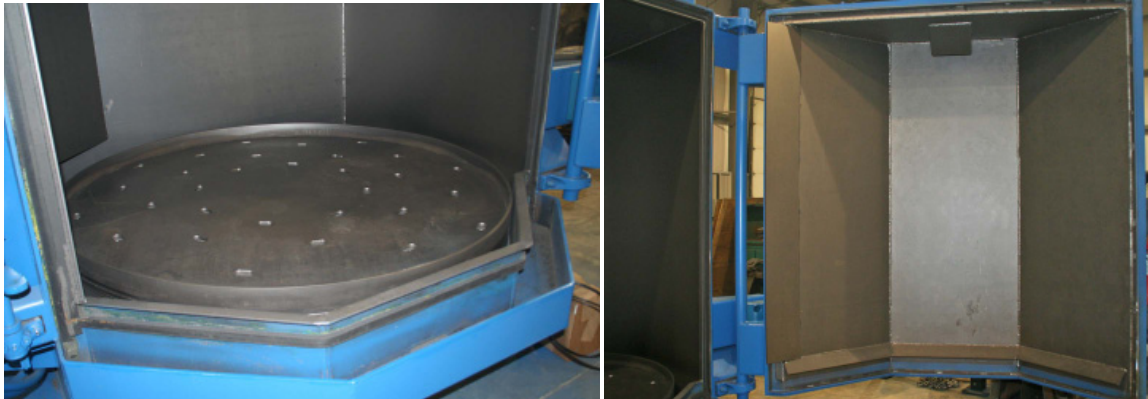
SHOT BLAST MACHINE SHOWING MANGANAL TABLE LINER, TABLE RING, AND WALL LINERS
