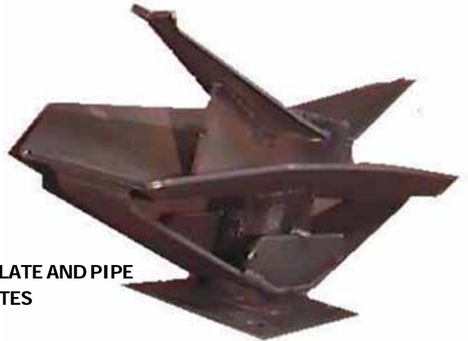
1/2" MANGAL FIXTURE HOLDS PARTS IN PLACE FOR ACCURATE BLAST CLEANING
