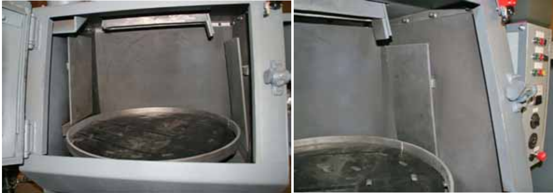
SHOT BLAST MACHINES SHOWING MANGANAL TABLE LINER, TABLE RING, HANGING LINERS, AND BLAST WHEEL HOUSING
