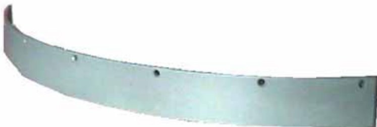
1/2" MANGAL PLATE ROLLED TO MATCH THE CAROUSEL TABLE INSIDE OF A SHOT BLAST CABINET. THE HOLES ARE COUNTERSUNK TO ALLOW THE ATTACHMENT HARDWARE TO BE FLUSH WITH SURFACE OF THE WEAR PLATE
