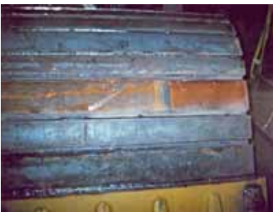
Manganal Wear Bars on Bottom of Excavator Bucket
