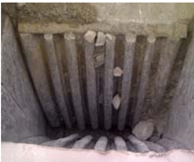
Crusher Jaw Repointed with 2-1/2" Manganese Round Bars after 1-year in service
