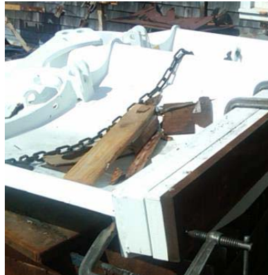
Stulz 8000 Grapple Front and Back Tips 2-1/2 years in Metal Recycling Plant
