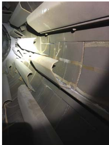
Stulz 8000 Drum Liner after an entire season, Edges Still Sharp!
