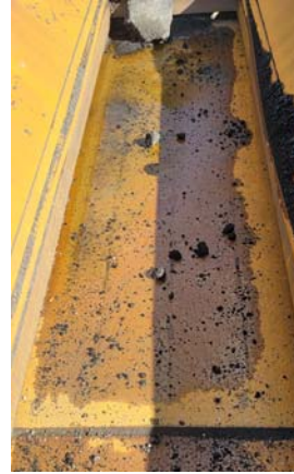
Feeder Floor (left) in 1/2" Stulz 4800 after 3 years, no wear, sharp edges still!
