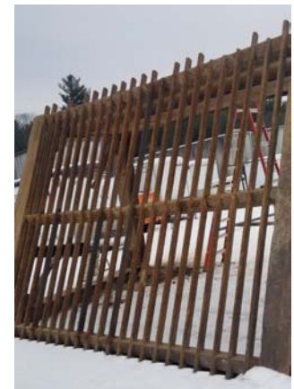
Rebuilt Screener with 901 Grouser bars
