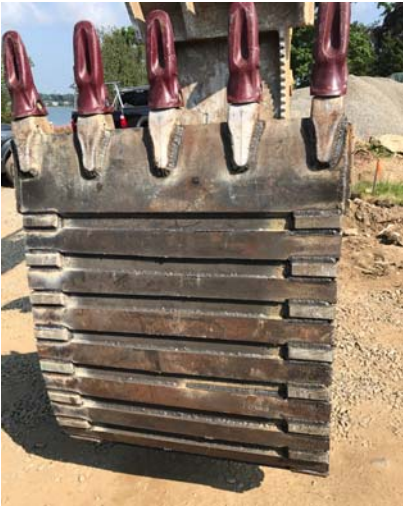
3/4" Wear Bars after 1yr digging through 7,000 yards of rock and 7 foundations!
