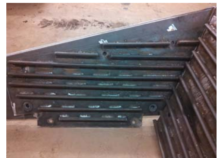
Stulz-Grouser Bars used to trap material in Feed Hopper
