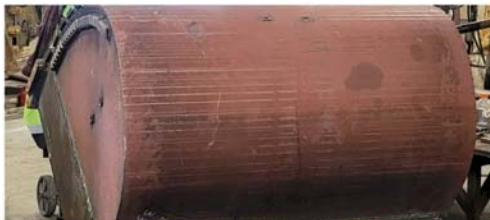
Stulz 8000 Formed to Full C Floor, Cheek Plates, Outside Cheek Liners, and custom-cut Wear Bars
