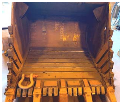
Excavator with custom-formed Stulz 8000 Floor reinforced with cut 8000 Bars & Blocks
