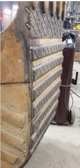
1/2" Wear Bars hardfaced with Stulz XL after 2 seasons
