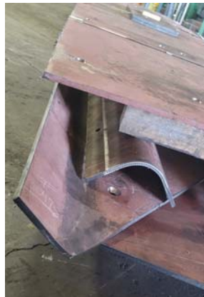
Stulz 4800 Forms to 90° & 45° Bends, and easily allows Threaded, Countersunk, or Counter-bored Holes, while still outperforming any water-quenched steels!
