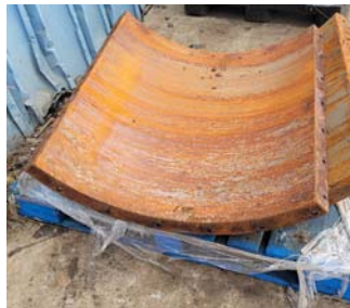
Hadfield-Grade Manganese Anvil in Metal Recycling Plant Outlasted OEM 4 to 1
