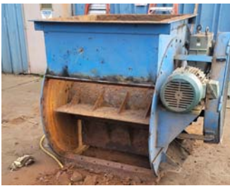
Crusher Jaw Repointed with 2-1/2" Manganese Round Bars after 1-year in service
