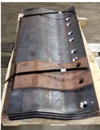
Designed to replace 5 pieces 10 Countersunk holes, 3 bends!
