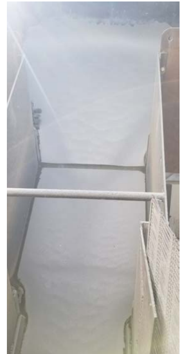
Extreme-Wear Chute - Manganese on top half, Complex-Carbide on bottom
