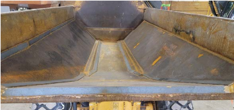
We measure and diagram any job! Cat Articulated Rock Body in Stulz 8000, Cut to Fit.
