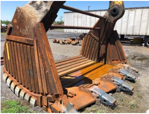
PC400 Bucket lined with Stulz 8000 Bars at a Coal Mine
