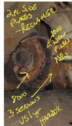
Reclaimer wall Stulz 8000 vs Hardox 450 3 years vs 1 year!
