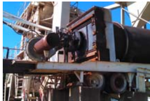
Stulz 8000 Burner Wall, Burner Hood and Burner Ring in Batch Plant No Warpage!
