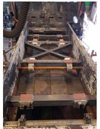
Stulz 8000 used to protect paddle arms and interior on a Roadtec Conveyor
