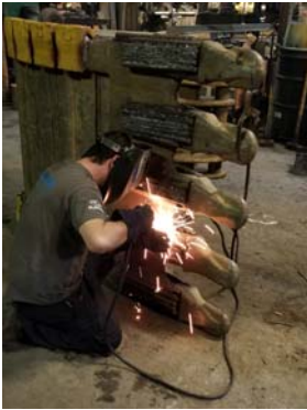
Manganese bars welded on shanks with Stulz XL
