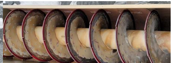
High Grinding Application Stulz 8000 in Screw Conveyor
