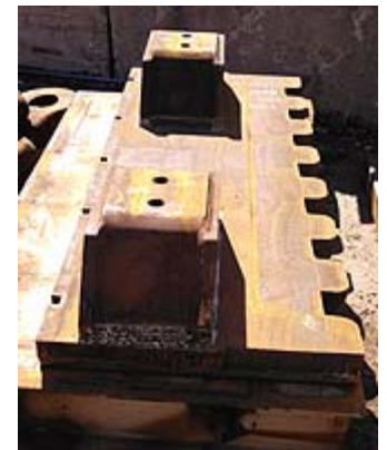
Hadfield-Grade Manganese Anvil in Metal Recycling Plant Outlasted OEM 4 to 1
