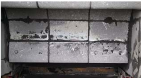
Manganese Impact Plates After 120,000 tons of recycled asphalt OEM only lasted 30,000
