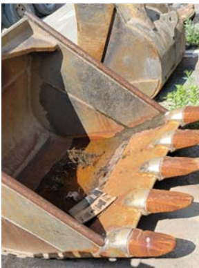
Manganese Round Bars, Inside Formed Liner, and Outside Cheeks after 24 months in Shot Rock
