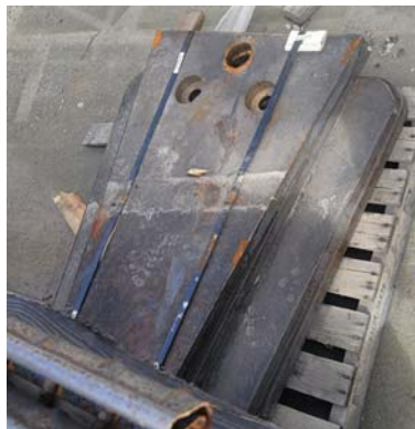
Manganese Cheek Plates for Metso 120 Crusher Holes Custom-Machined to fit socket head for quick changing!
