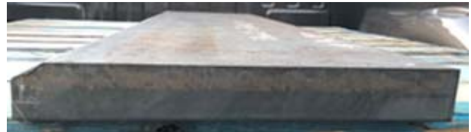
Custom-designed Bevel Lip to fit Shank
