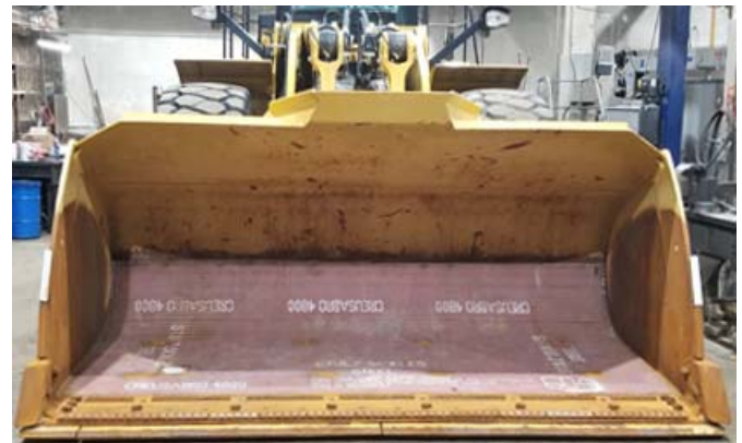
980M Liner Formed To Fit in 4800
