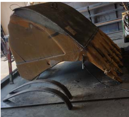
Stulz 8000 Formed Floor & Skis Custom bars & Cheek Liners
