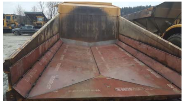
Cat 773B Rock Body lined with Stulz 4800 cut per diagram
