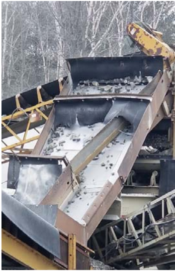
3/8" Stulz 8000 Chute wears differently. We designed interlocking pieces for maximum wear life. Customer welded studs on back for easy replacement.
