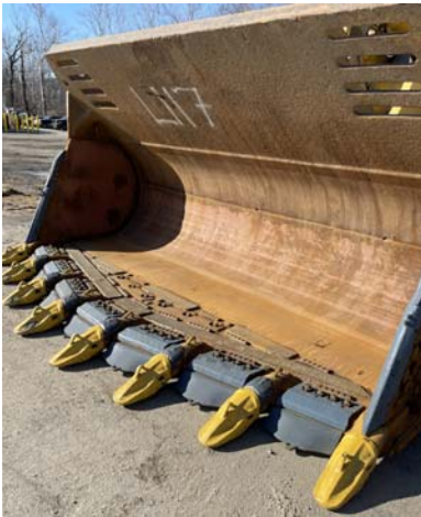
5/8" Stulz 8000 Formed for Quarry in Pennsylvania
