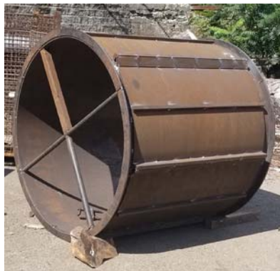
Stulz-Sickles Specializes in manufacturing Hadfield-grade Manganese Magnet Shells to your specifications that far outlast standard OEM. We also fabricate high-wear collar flanges.
