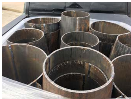
Stulz 8000 Cone Lips welded to Stulz 4800 Cylinders for loading Sand in Railcars
