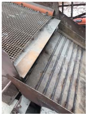
1" Hex Grouser over Stulz 4800 Trips media & creates material on material
