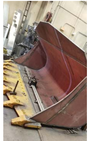
Plus Cheeks, Cheek Liners and Side Cutters. Formed Back Top Plate in 1/2" Stulz 4800
