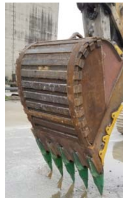
Manganese Bars, Rolled Skis, Cheek Liners and Corner pucks for Severe Applications
