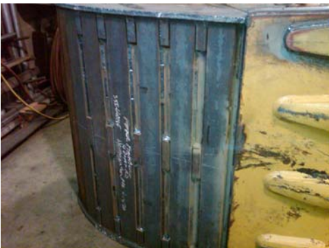
Wear Bars reinforcing an excavator bucket
