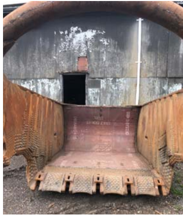
Dragline Liner in Stulz 4800
